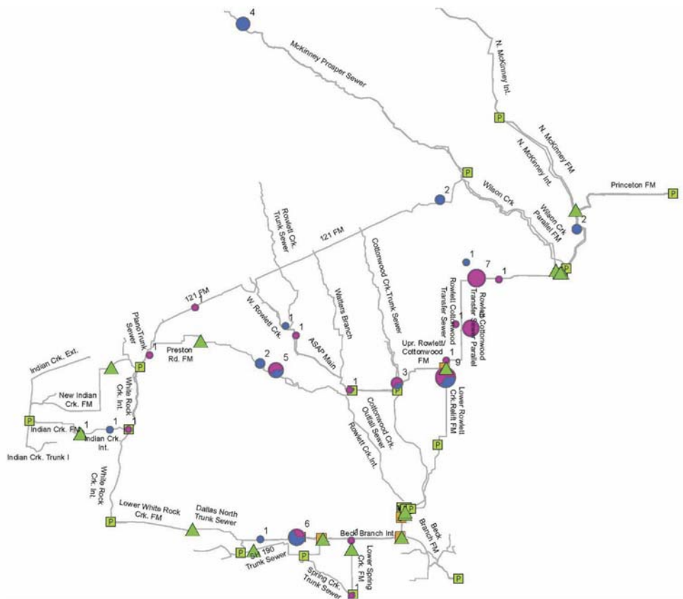
Figure 3. North Texas Municipal Water District Odor Complaints and Force Main Discharge Locations
